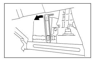
Lift the top tab on the cover to remove the filter cover.
